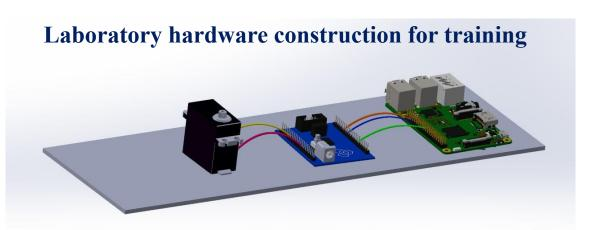
Right to Left: Raspberry Pi, FPGA demo board, servo motor as a peripheral device
