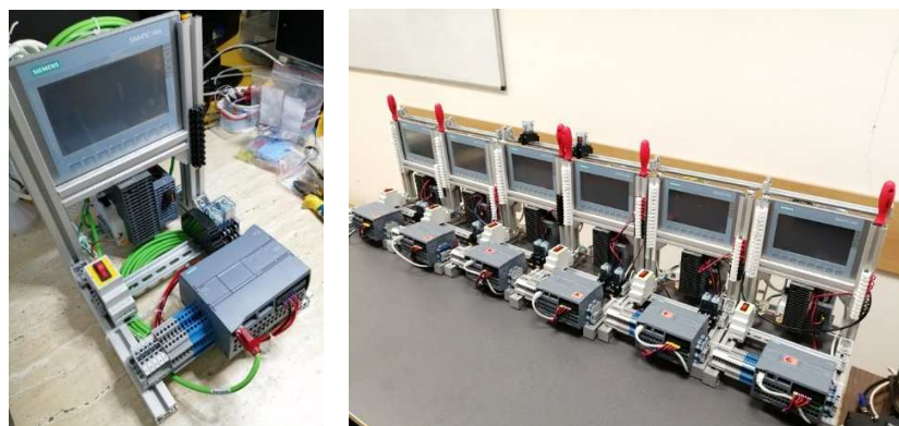
Fig. 1. Training stands with programmable logic controllers
