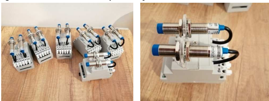
Fig. 4. Modules with inductive sensors
